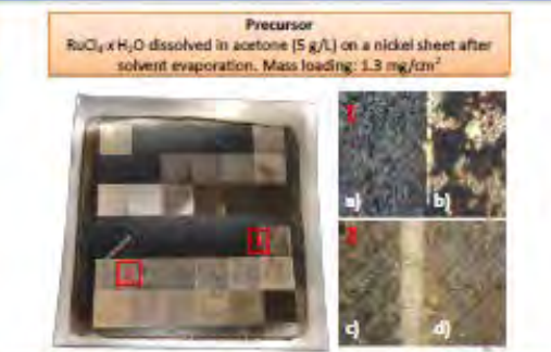
Fig. 5: a) 30% pumping power: closed surface, dark areas of dissociated RuCl 3 b) 30.5%: islands of dissociated RuCl 3 c) 31%: remelted nickel, inclusions of RuO 2 d) 31.5%: remelted nickel, removed inclusions.
