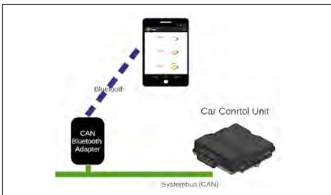
Figure 4: System overview of the wireless system
